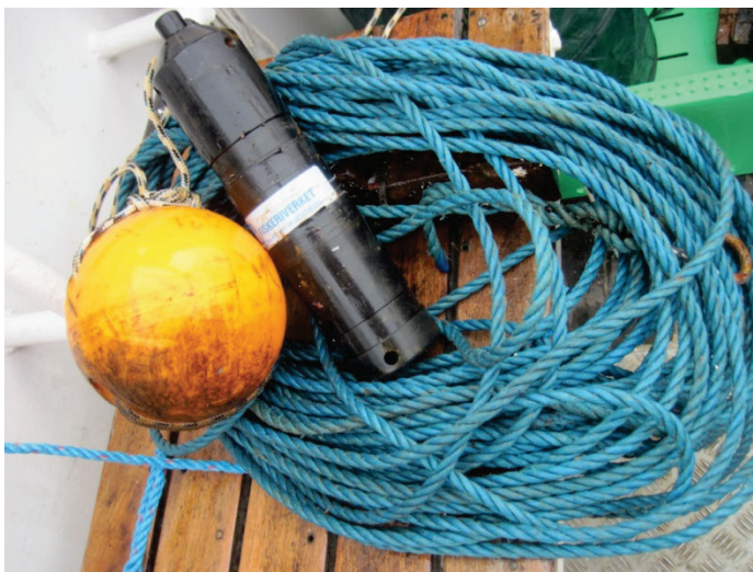
Figure 44. A hydrophone with the attached buoy and the line stretched along the bottom to allow recovery of the device by dragging (photo Ingvar Lagenfelt).
