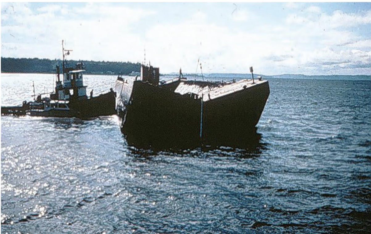
Figur 3. Example of sand capping using a bottom-discharging barge towed by a tugboat (image from Bailey et al. 2005).
