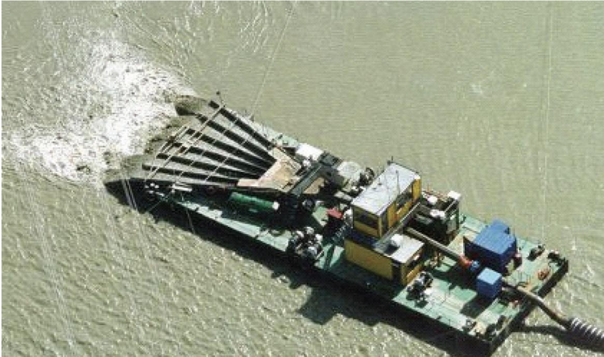
Figur 7. Automated hydraulic capping barge (picture from Bailey m.fl. 2005).
