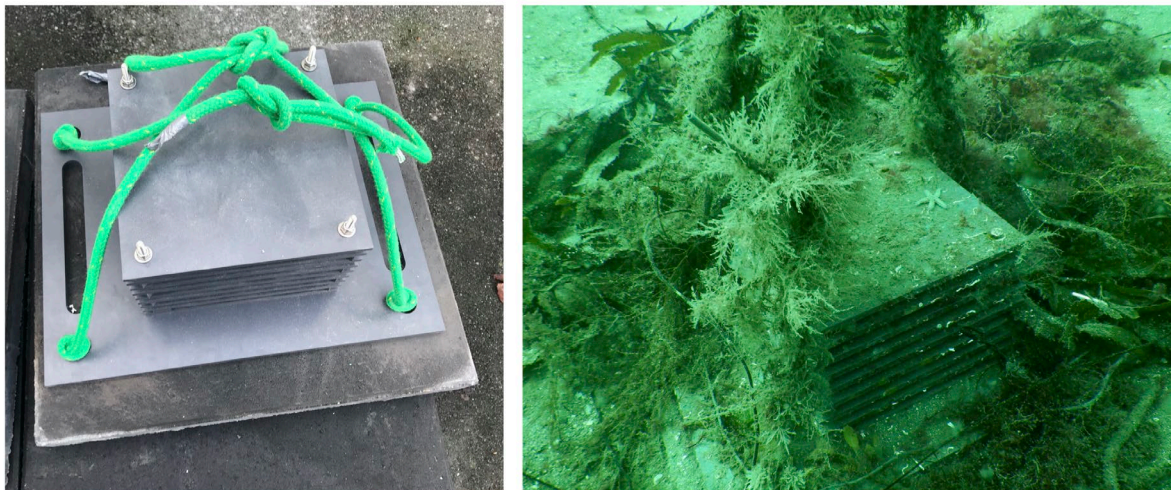
Figure 1. Left: Assembled ARMS panels before deployment at sampling site, with a concrete slab attached to the bottom plate. Right: ARMS photographed on the seafloor 12 months after deployment. Photo: Per Sundberg (left), Matthias Obst (right)
