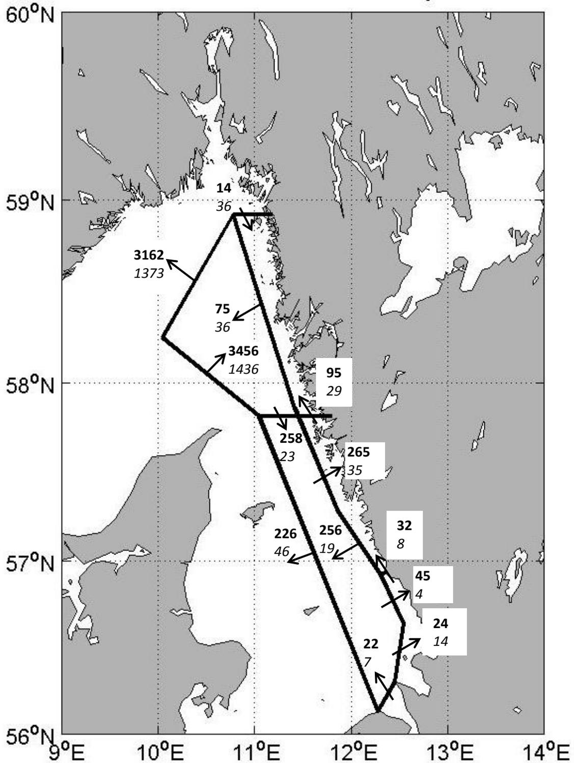
Figure 5. Mean annual nitrate transports ( $\text{kton yr}^{-1}$ ) 2007-2011 (bold) and standard deviation (italic) between the years. Unit:  $\text{kton}=10^6 \text{ kg}$ .
