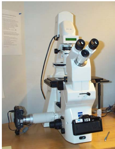
Fig. 5 An inverted microscope suitable for analysing phytoplankton using the Utermöhl method. Photo by Bengt Karlson.
