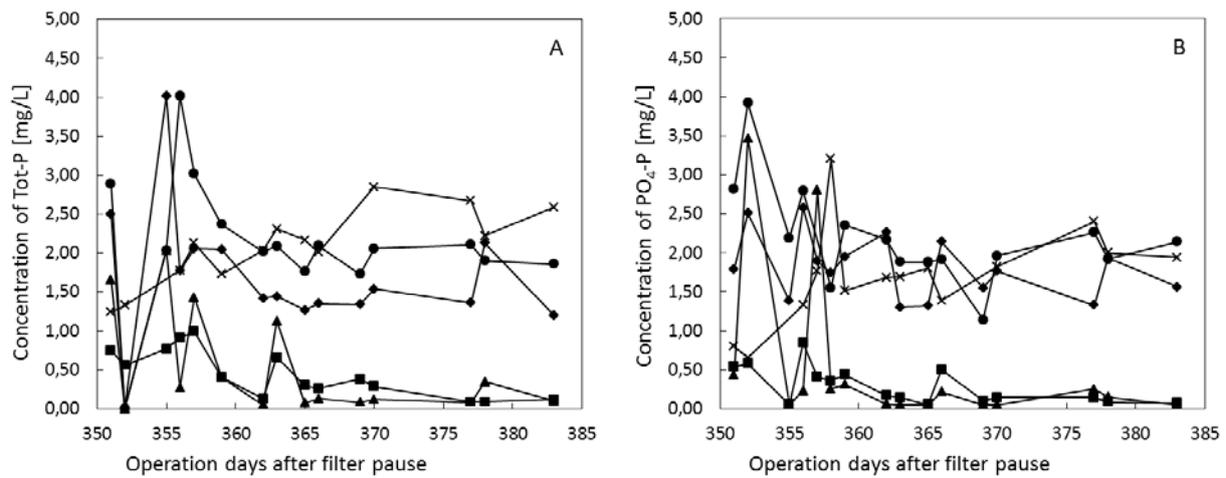
**Figure 7.** A) Total phosphorus (Tot-P) concentration and B)  $\text{PO}_4\text{-P}$  concentration in the influent (x) and filter effluent after re-start of the filters following a pause in operation: unimpregnated biochar (UBC; ●), CaO-impregnated biochar (CBC; ■),  $\text{FeCl}_3$ -impregnated biochar (FBC; ▲) and biochar mixed with Polonite (PBC; ◆)
