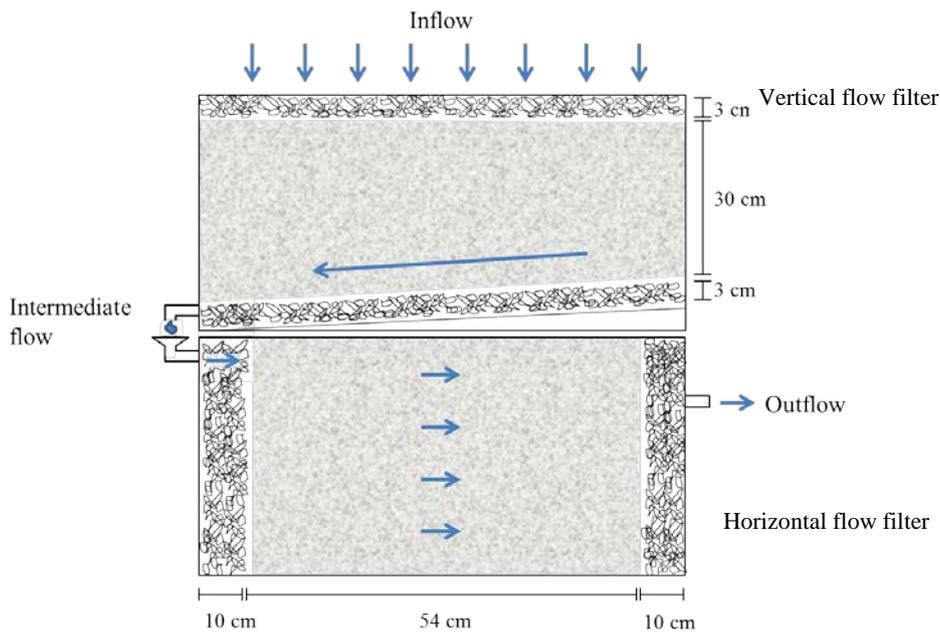
**Figure 8.** Combined aerobic vertical flow and anaerobic horizontal flow biochar filter unit for wastewater nitrogen removal. The material in the filter was biochar made from hardwood biomass. The figure is obtained from Stenström (2017).
