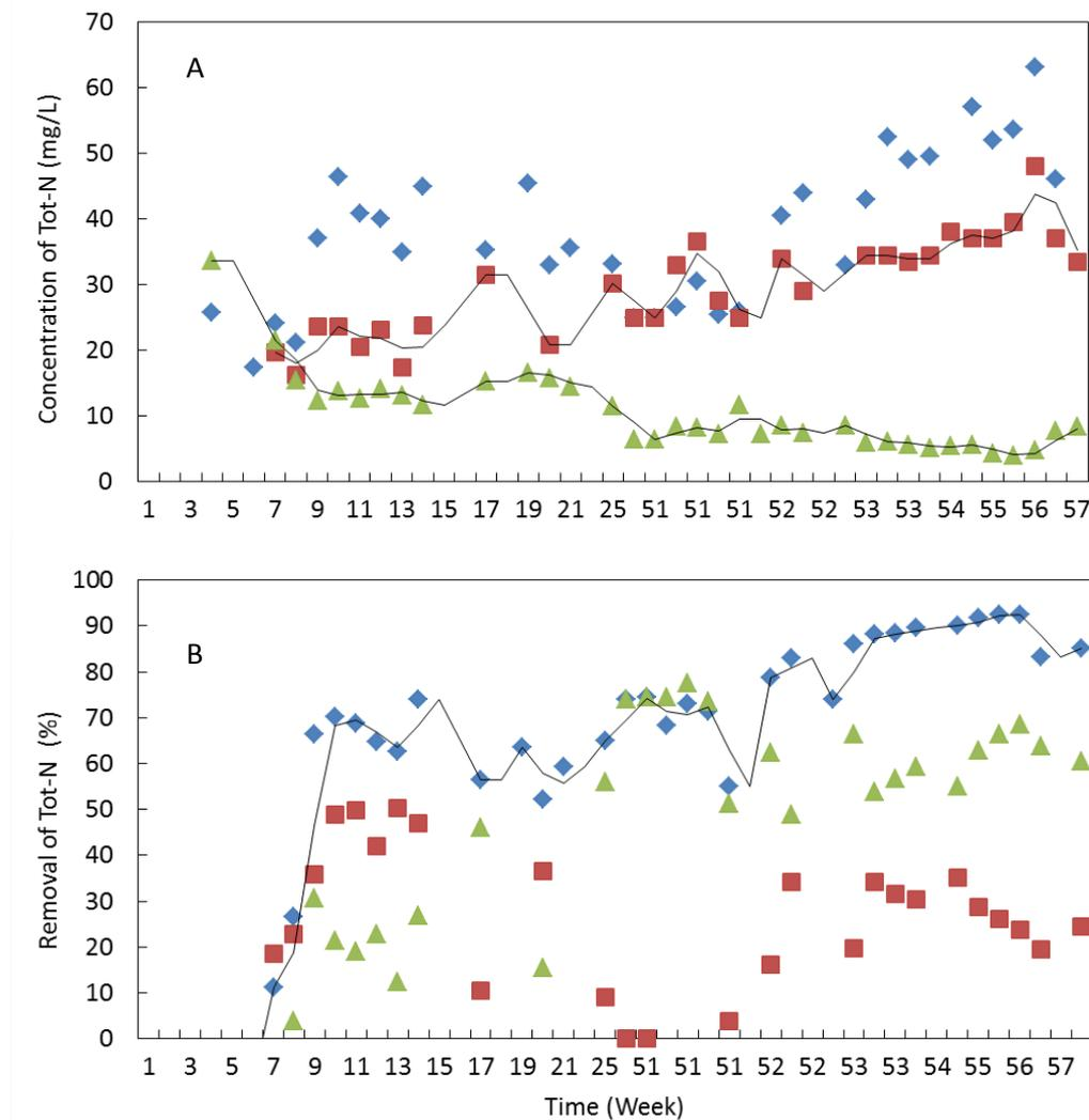
**Figure 10.** Weekly variation in A) total nitrogen (Tot-N) concentration and B) Tot-N removal in the vertical flow filter section (■), the horizontal flow filter section (▲) and the combined filter system (◆) during 57 weeks of operation.
