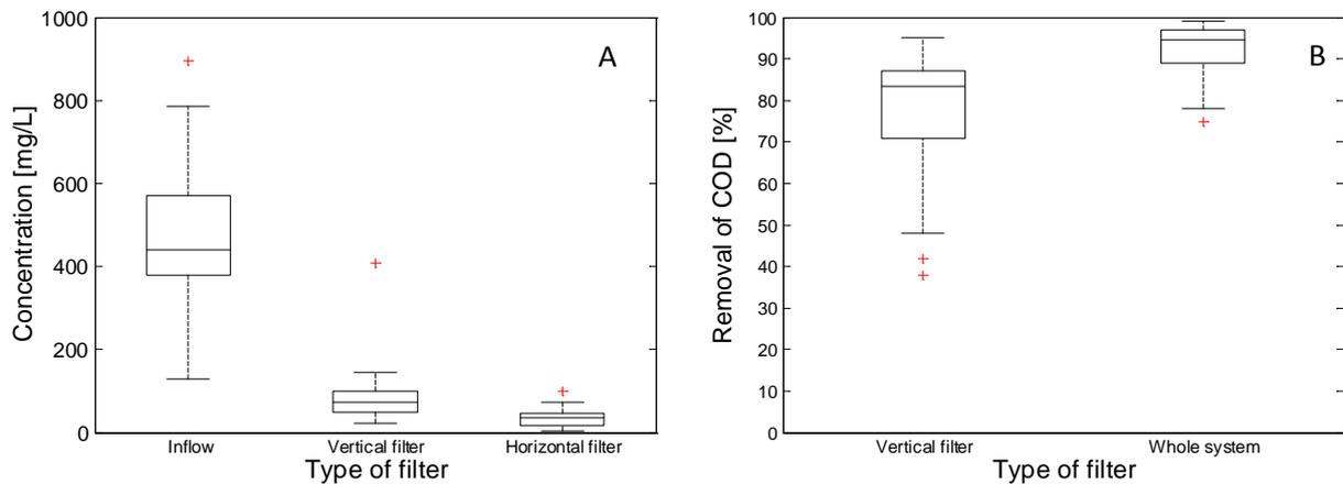
**Figure 9.** Box plots of A) the concentration of chemical oxygen demand (COD) and B) the percentage removal of COD in the vertical flow filter and in the whole system (vertical + horizontal filters). The box is the quartiles, with the horizontal line in the box showing the median. Max and min values are the whiskers and outliers are presented as red crosses
