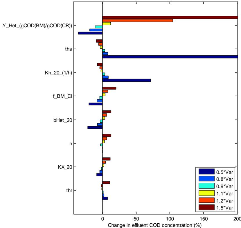
**Figure 18.** Sensitivity of the simulated chemical oxygen demand (COD) concentration in biochar filters in response to changes in model input parameters in the model. Data reported by Ciuk Karlsson (2015).
