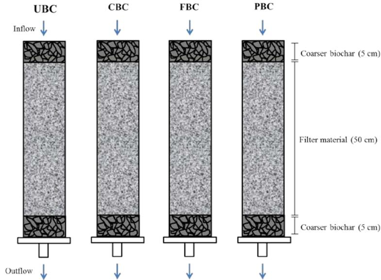
**Figure 1.** Experimental set-up used for column filters filled with unimpregnated biochar (UBC), biochar impregnated with calcium oxide (CBC), biochar impregnated with ferric chloride (FBC) and biochar mixed with Polonite (PBC). Figure is obtained from Stenström (2017).
