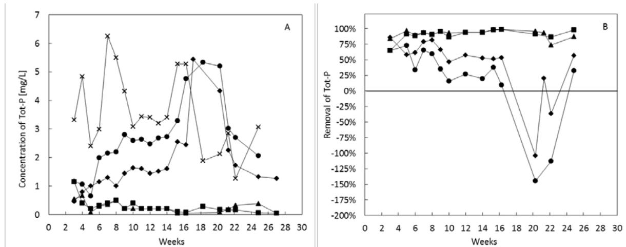
**Figure 4.** A) Total phosphorus (Tot-P) concentration in the influent (x) and in the effluent from the untreated biochar filter (UBC; ●), CaO-impregnated biochar filter (CBC; ■),  $\text{FeCl}_3$ -impregnated biochar filter (FBC; ▲) and biochar filter mixed with Polonite (PBC; ◆). B) Removal efficiency of Tot-P in UBC (●), CBC (■), FBC (▲) and PBC (◆).
