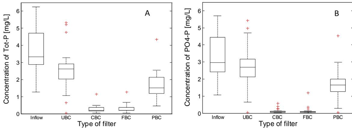
**Figure 6.** Boxplots of A) Total phosphorus (Tot-P) concentration and B) phosphate-P (PO<sub>4</sub>-P) concentration in the unimpregnated biochar filter (UBC), CaO-impregnated biochar filter (CBC), FeCl<sub>3</sub>-impregnated biochar filter (FBC) and biochar filter mixed with Polonite (PBC). The box is the quartiles of the data set and the medians are shown as a straight line in the box. Max and min values are the whiskers and outliers are shown as red crosses.
