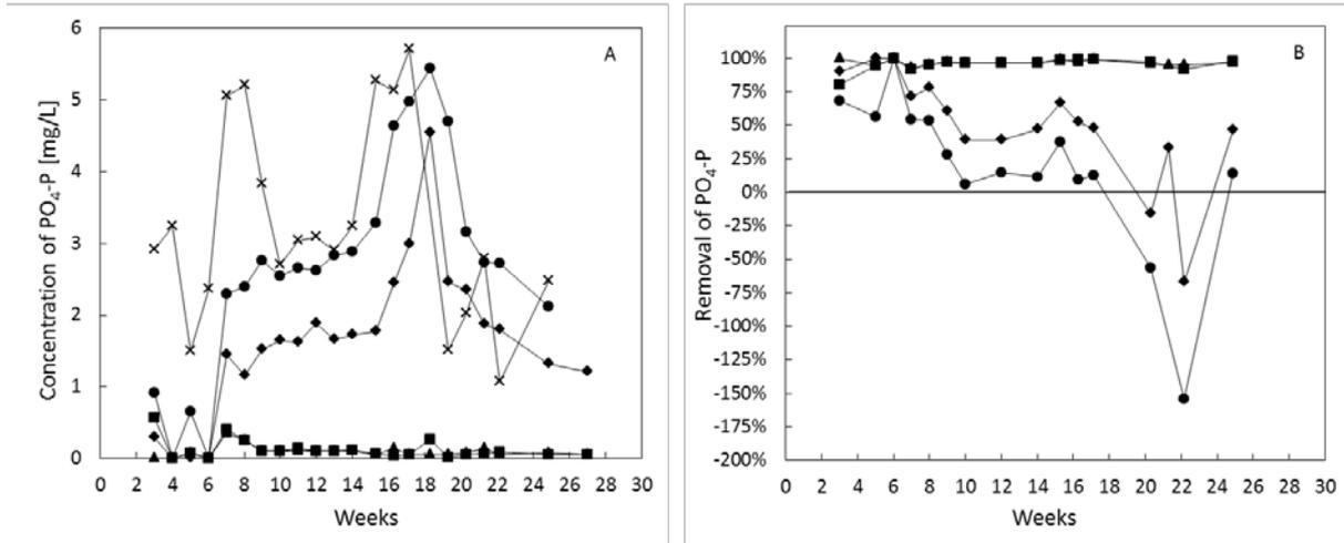
**Figure 5.** A) Phosphate phosphorus (PO<sub>4</sub>-P) concentration in the influent (x) and effluent from the FeCl<sub>3</sub>-impregnated biochar filter (FBC; ▲), CaO-impregnated biochar filter (CBC; ■), biochar filter mixed with Polonite (PBC; ◆) and unimpregnated biochar filter (UBC; ●). B) Removal efficiency of Tot-P in FBC (▲), CBC (■), PBC (◆) and UBC (●) filters.
