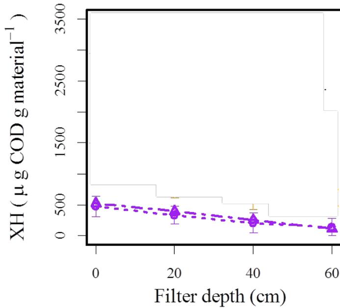
**Figure 14.** Observed (●) and simulated (▲) concentration of heterotrophic microorganisms (XH) in biochar filters at depths 0, 20, 40 and 60 cm, with hydraulic loading rate  $32 \text{ L m}^{-2} \text{ day}^{-1}$  and organic loading rate  $14 \text{ g BOD}_5 \text{ m}^{-2} \text{ day}^{-1}$ . The points show mean values determined during a 5-day simulation and the error bars display standard deviation.
