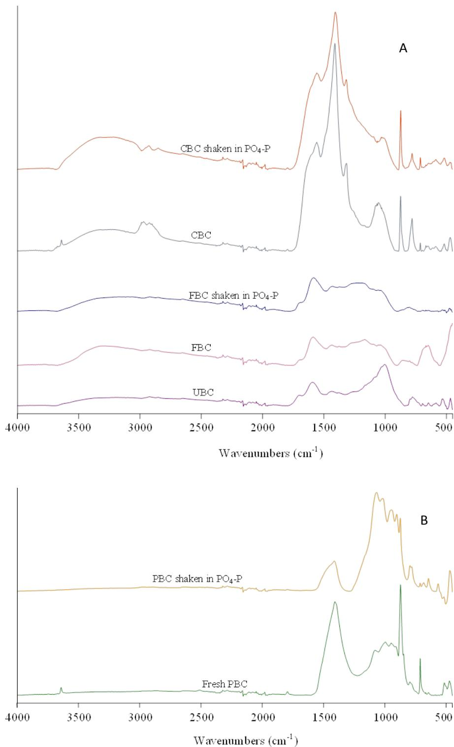
**Figure 2.** Fourier transform infrared (FTIR spectra) of: A) unimpregnated biochar (UBC, purple), biochar impregnated with calcium oxide (CBC, orange) and biochar impregnated with ferric chloride (FBC, blue); and B) biochar mixed with Polonite (PBC).
