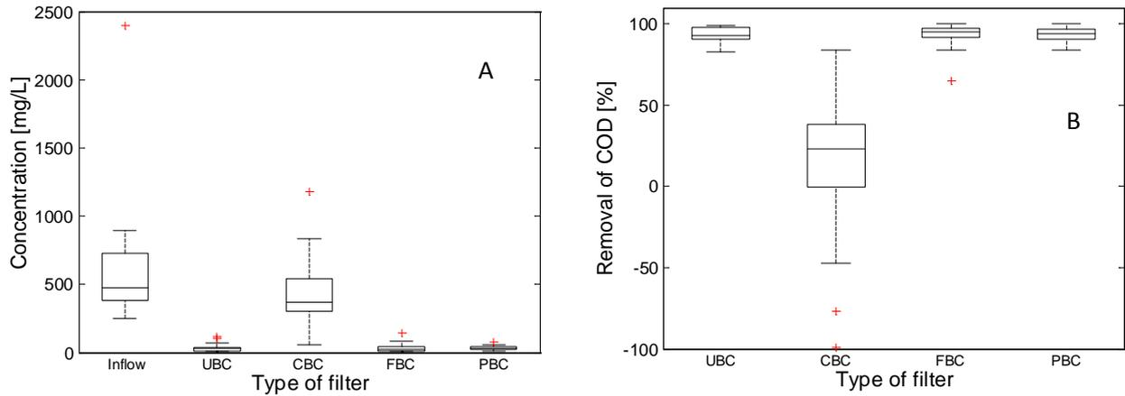
**Figure 3.** Boxplots of A) chemical oxygen demand (COD) concentration and B) COD removal in the unimpregnated biochar filter (UBC), CaO-impregnated biochar filter (CBC), FeCl<sub>3</sub>-impregnated biochar filter (FBC) and biochar filter mixed with Polonite (PBC). The box is the quartiles of the data set and the medians are shown as a straight line in the box. Max and min values are the whiskers and outliers are shown as red crosses.
