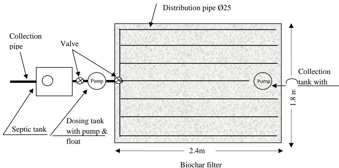
**Figure 19.** Schematic diagram of the biochar treatment system used for a single-family household, including septic tank, dosing equipment and biochar filter (Dalahmeh, 2016).
