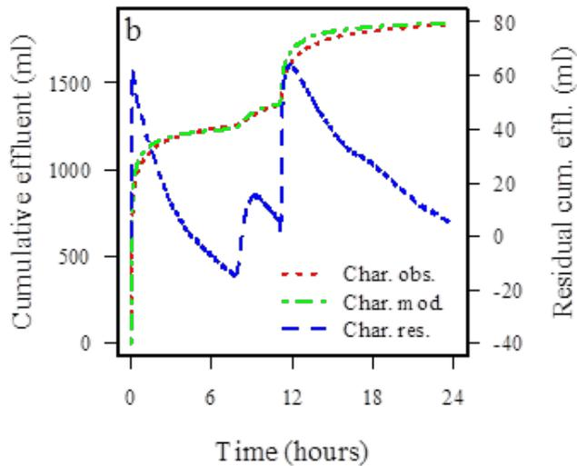
**Figure 13.** Observed (-----) and simulated (-----) cumulative effluent (mL) in the biochar filter as a function of time (hours) and calculated residual cumulative effluent (-----) of simulated flow, compared with observed cumulative effluent data at a hydraulic loading rate of  $32 \text{ L m}^{-2} \text{ day}^{-1}$ . These results are reported by Ciuk Karlsson (2015).
