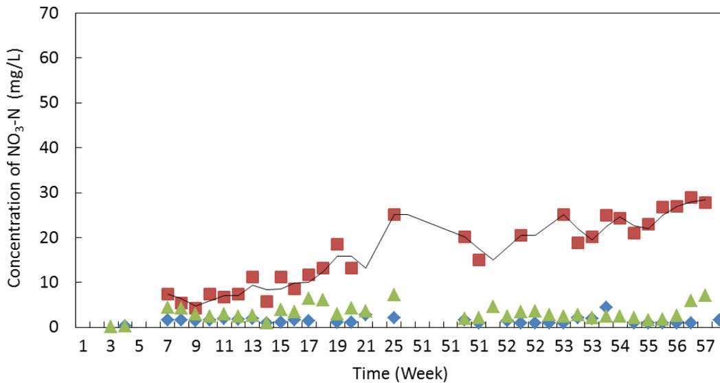
**Figure 12.** Weekly variation in nitrate-nitrogen ( $\text{NO}_3\text{-N}$ ) concentration in the vertical flow filter section (■), the horizontal flow filter section (▲) and the combined filter system (◆) during 57 weeks of operation.
