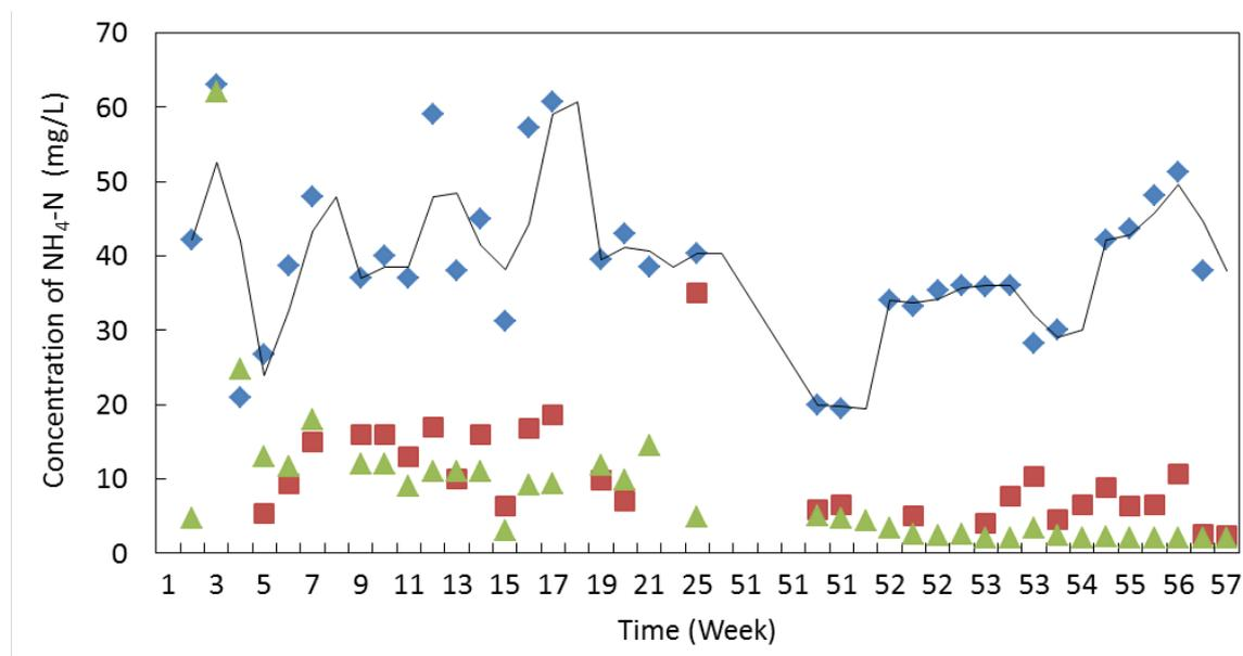
**Figure 11.** Weekly variation in ammonium-nitrogen ( $\text{NH}_4\text{-N}$ ) concentration in the vertical flow filter section (■), the horizontal flow filter section (▲) and the combined filter system (◆) during 57 weeks of operation.
